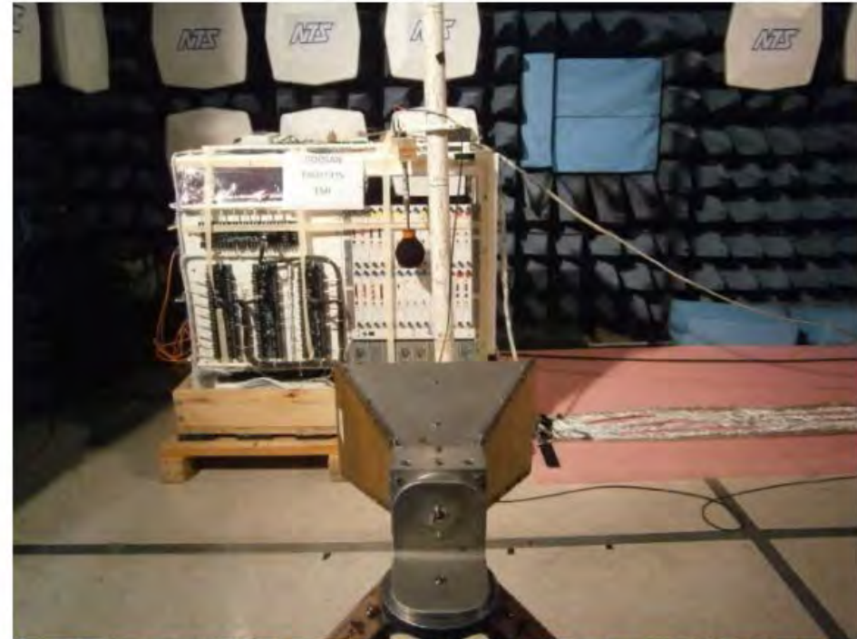
General Test Setup for RS103 from 8GHz - 10GHz, Vertical Front (right side of the EUT)
