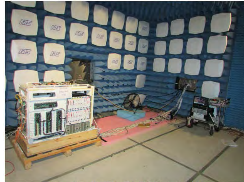
General Test Setup for CS101 120Hz – 150 kHz
