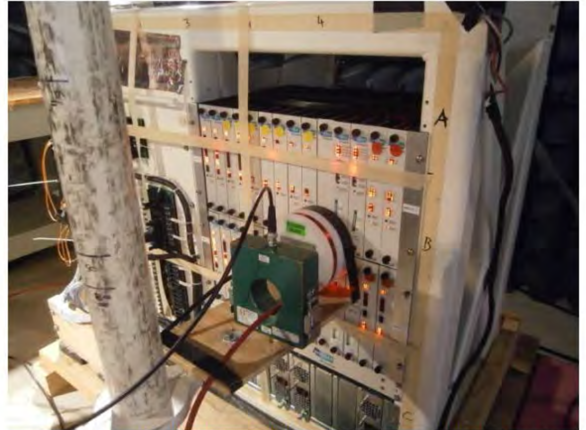
Test Setup for RS101, 30Hz – 100 kHz, Front of the EUT, Location B4
