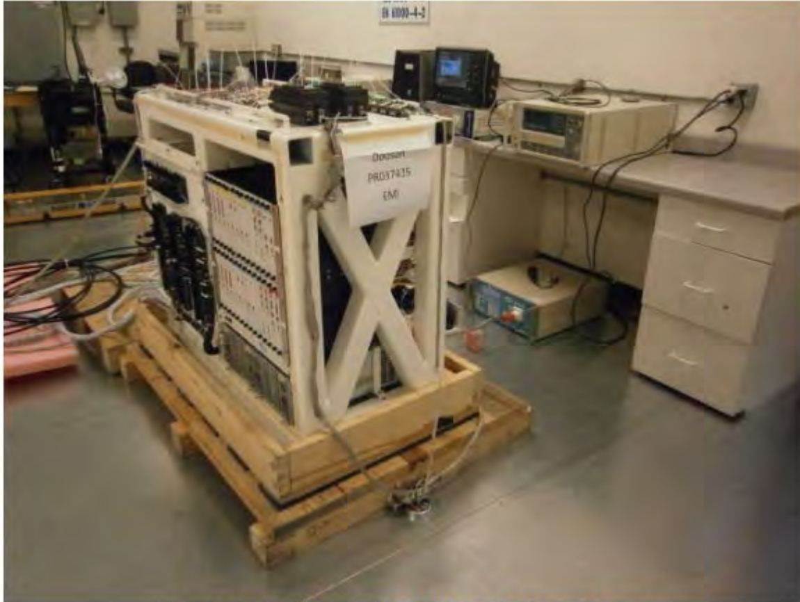
General Test Setup for EFT, AC Power Input
