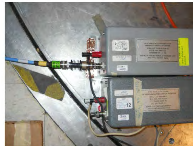
Line Test Setup for CE102
