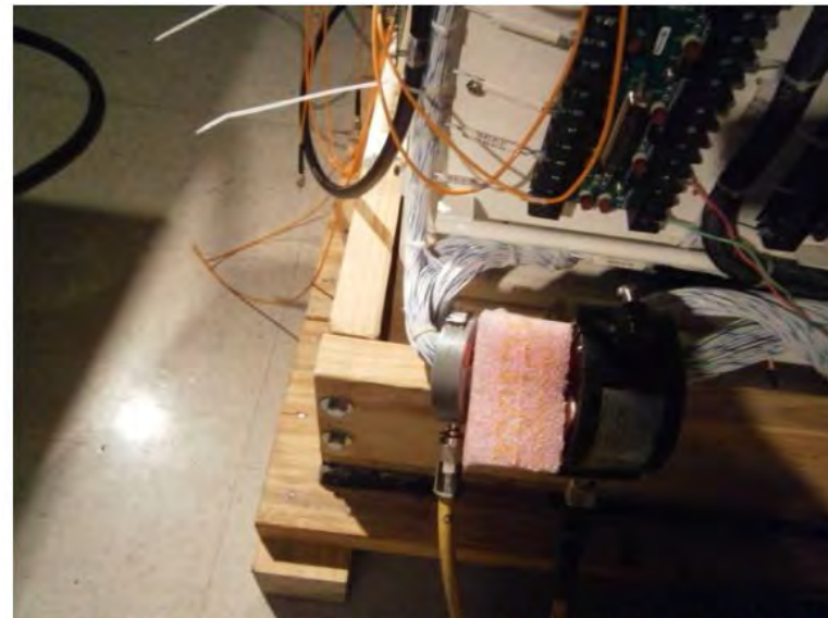
General Test Setup for CS114 from 10 kHz – 30MHz, Test on Signal Bundle 2
