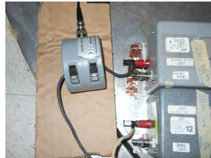
Line Test Setup for CE101
