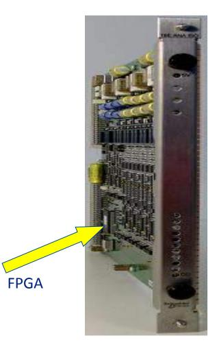
Previous analog board: 1 microprocessor + logic circuits; 6 analog channels per board
